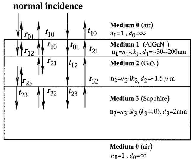
FIG. 1. Schematic diagram of the AlGaN/GaN/sapphire heterostructure and the reflection and transmission of the normal-incidence light in this multi-layered system.
