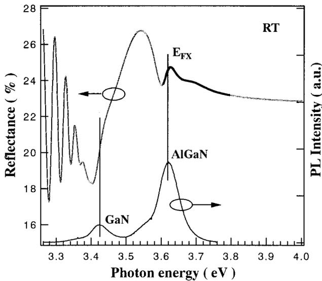
FIG. 7. A typical fitting curve of the experimental reflectance spectrum of the  $\text{Al}_{0.08}\text{Ga}_{0.92}\text{N}/\text{GaN}$  heterostructure with the AlGaN layer about 200 nm. The free exciton transition energy ( $E_{\text{FX}}^A$ ) obtained shows a good agreement with the peak energy of the PL spectrum.
