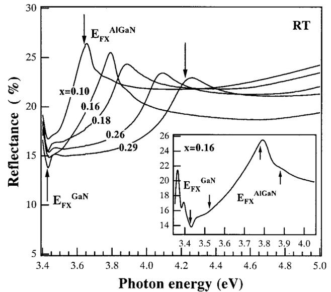
FIG. 6. Room temperature reflectance spectra of AlGaN (~30 nm)/GaN (~1500 nm) heterostructure samples with various Al mole fraction,  $x$ . The excitonic transition energies of GaN ( $E_{FX}^{GaN}$ ) and AlGaN ( $E_{FX}^{AlGaN}$ ) are marked by vertical arrows. The inset shows the spectrum of the  $x=0.16$  sample. Broad features ascribed to exciton-LO phonon interaction were observed at optical energies about 100 meV above the  $E_{FX}^{GaN}$  and  $E_{FX}^{AlGaN}$ , respectively.
