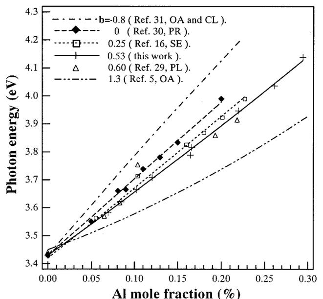
FIG. 8. Al composition dependence of the exciton transition energies derived from the reflectance measurement. Such dependencies of band gap energy derived from CL, OA, PL, PR, and spectroscopic ellipsometry (SE) methods in literature were shown together.
