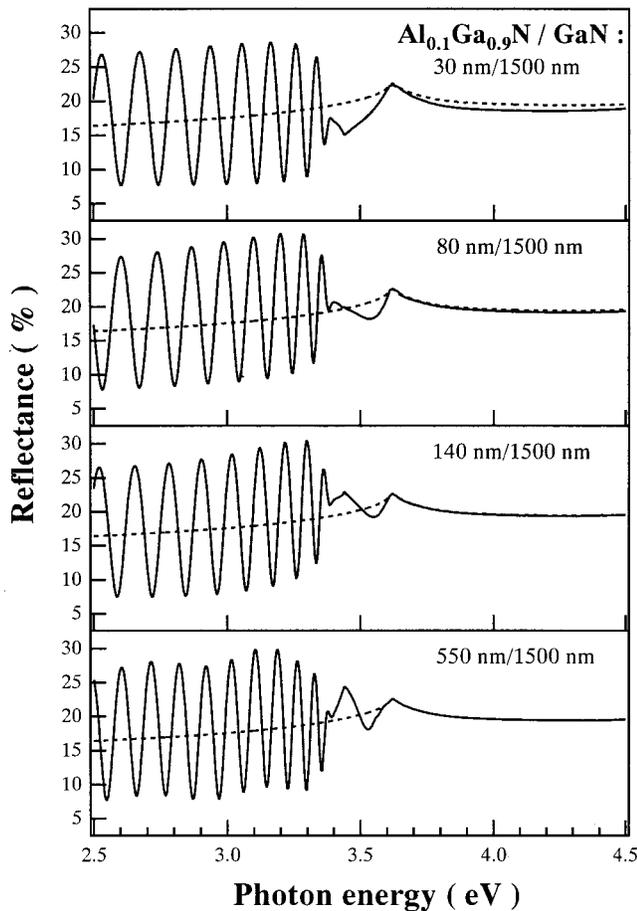
FIG. 5. Calculated reflectance spectra of  $R_{01}$  (dashed line) and  $R$  (solid line) with various thickness  $d_1$ . With the increase of  $d$ ,  $R_{01}$  shows a trend of agreement with  $R$  at the excitonic profile of AlGaN. It also shows the amplitude of  $R_{01}$  is a dominant part in that of  $R$ .
