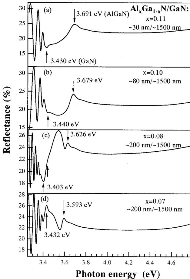
FIG. 3. Experimental reflectance spectra for  $\text{Al}_x\text{Ga}_{1-x}\text{N}/\text{GaN}/\text{sapphire}$  ( $x$  around 0.1) heterostructures with various thicknesses of AlGaIn layers ( $d_1$ ). The thickness values were measured by thickness monitor in the growth process of epilayers. It shows that the excitonic profile of GaN is hidden in interference fringes when  $d_1$  is about 200 nm.
