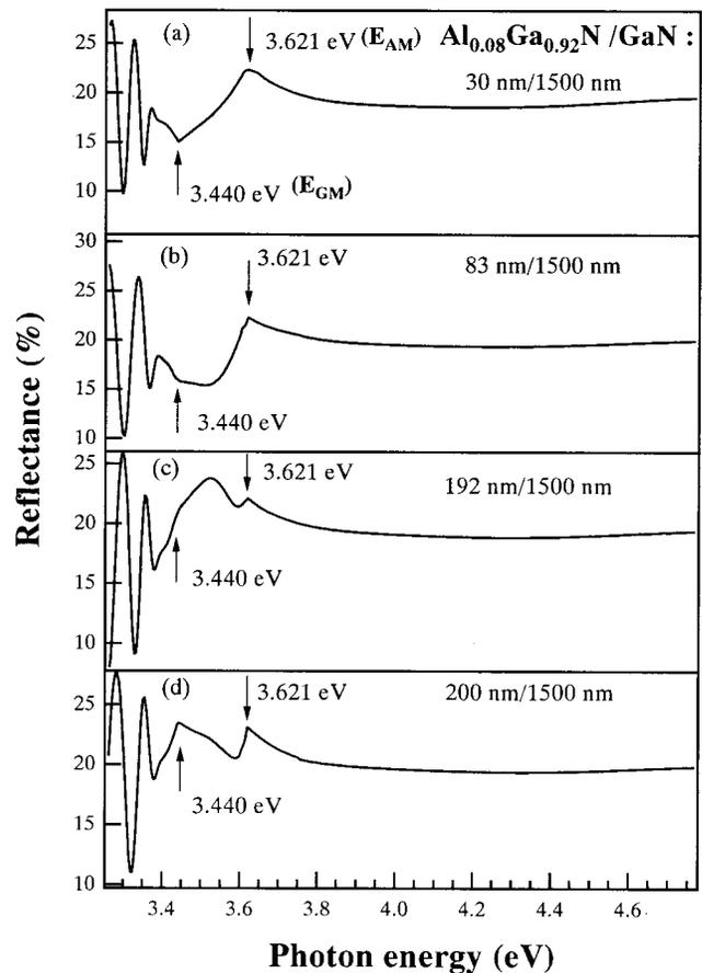
FIG. 4. Calculated reflectance spectra for  $\text{Al}_{0.08}\text{Ga}_{0.92}\text{N}/\text{GaN}/\text{sapphire}$  heterostructures with thickness ( $d_1$ ) changes corresponding to that in Fig. 3. The line shape of region (b) shows the changes in agreement with that in Fig. 3, while the energy location of  $E_{AM}$  (3.621 eV) are not shifted.
