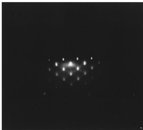
FIG. 1. RHEED pattern obtained from an as-deposited 20 nm GaAs nucleation layer on a Si/porous Si/Si substrate along a  $\langle 110 \rangle$  azimuth.
