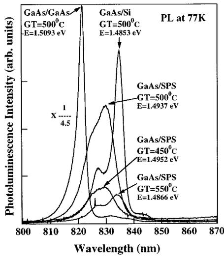
FIG. 3. 77 K photoluminescence of a CBE-grown GaAs epilayer on GaAs, Si, and Si/porous Si/Si substrates.
