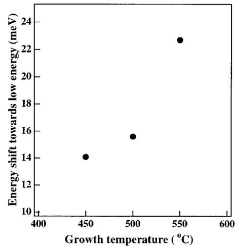
FIG. 4. Energy shift towards the low energy region in the growth of GaAs on a Si/porous Si/Si substrate when compared to CBE-grown GaAs/GaAs at 500 °C.
