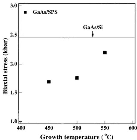
FIG. 5. Variation of biaxial tensile stress ( $X$ ) due to GaAs epilayer growth temperature.
