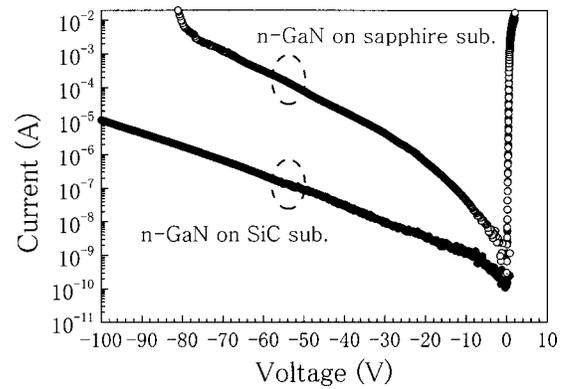
FIG. 3.  $\log(I)$ - $V$  characteristics of Ni/Au Schottky contacts on *n*-GaN grown on sapphire and SiC substrates.
