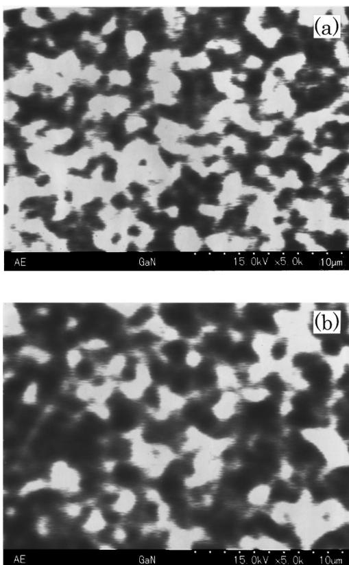
FIG. 5. EBIC images of Schottky diodes; (a) *n*-GaN grown on SiC substrate, and (b) *n*-GaN grown on sapphire.
