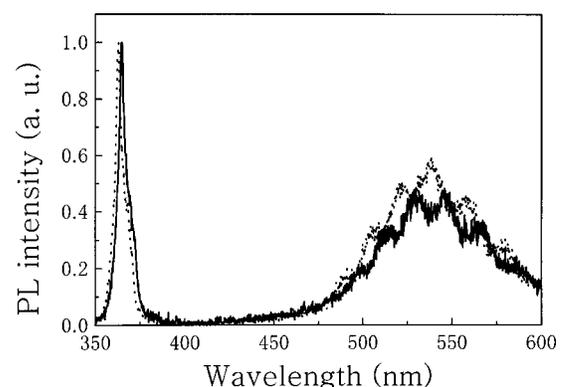
FIG. 1. Room temperature PL spectra of *n*-GaN grown on sapphire (dash line) and SiC substrates (solid line).
