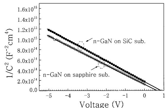
FIG. 4.  $C$ - $V$  characteristics of Ni/Au Schottky contacts on *n*-GaN grown on sapphire and SiC substrates.
