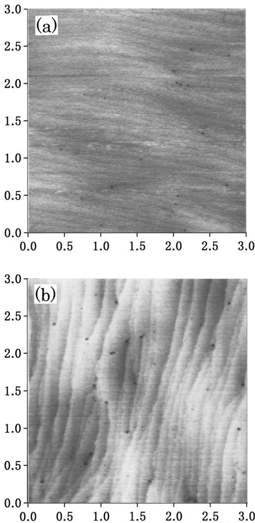
FIG. 2. AFM images of *n*-GaN surfaces in a  $3 \times 3 \mu\text{m}^2$  area; (a) *n*-GaN grown on SiC substrate, and (b) *n*-GaN grown on sapphire.
