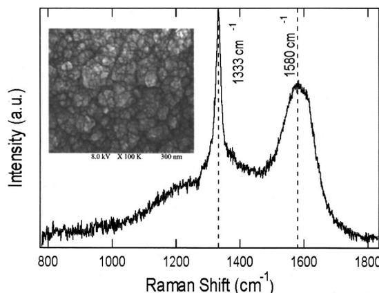
FIG. 4. UV Raman spectrum taken at 257 nm of an NCD sample. Inset is a high resolution SEM micrograph of the sample.
