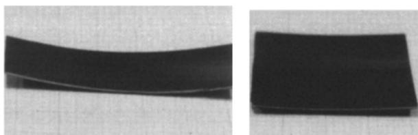
FIG. 2. Two visibly bent silicon samples after deposition because of high compressive stress in the carbon films deposited on them. The film is at the bottom side in the photographs.
