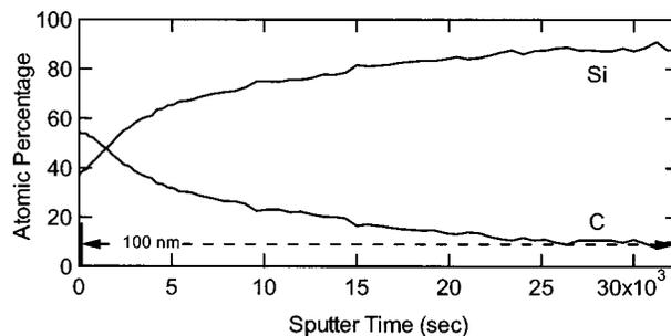
FIG. 3. XPS depth profile of a sample. The depth was estimated from stylus measurement on post-measured (sputtered) sample.
