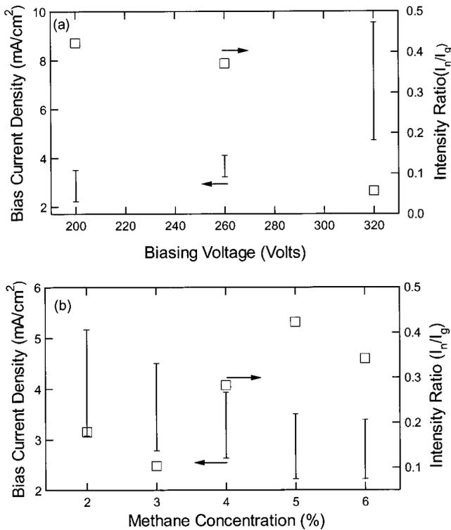
FIG. 5. Plots of BCD and the ratio of intensities of the Raman feature at  $1150\text{ cm}^{-1}$  (in visible Raman spectra) to graphitic G band ( $I_n/I_g$ ) as a function of (a) biasing voltage and (b) methane concentration. The bars indicate the range of variation of the BCD from start to end.
