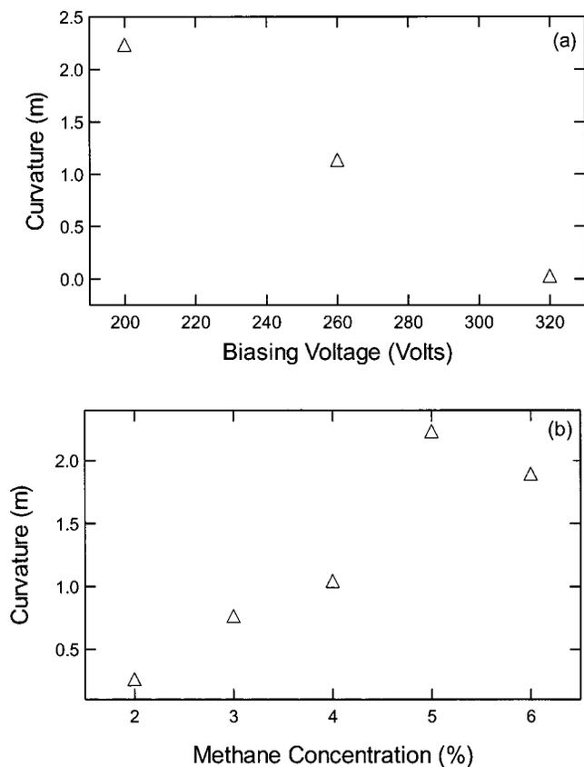
FIG. 1. Plots of radius of curvature as a function of (a) biasing voltage and (b) methane concentration.
