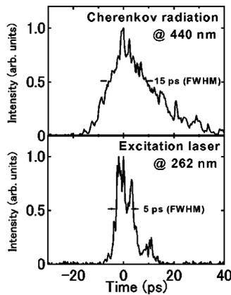
FIG. 2. Time profiles of Cherenkov radiation induced by the electron pulsed beam and the 262 nm laser pulse for excitation of photocathode or sample, measured by a spectrograph and a streak camera.
