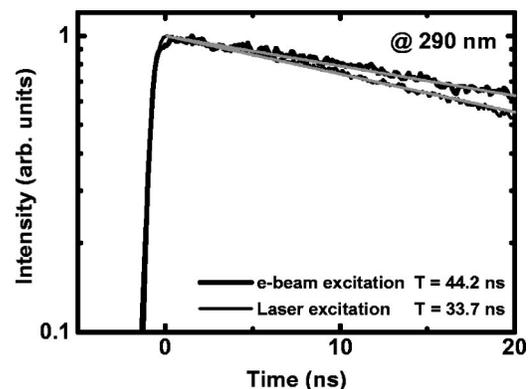
FIG. 5. Fluorescence decay curves of Ce:LiCAF excited by e-beam and by 262 nm pulse measured around 290 nm. The solid lines indicate the convolution curves with fixed lifetimes, 44.2 ns for e-beam and 33.7 ns for 262 nm. The lifetime from e-beam excitation was slightly longer than that from laser excitation.
