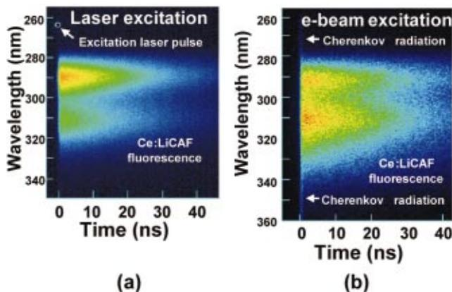
FIG. 3. (Color) Streak camera images of the fluorescence from Ce:LiCAF excited (a) by 262-nm pulse and (b) by electron pulse. In the case of electron pulse excitation, a broadband, short-duration Cherenkov radiation is clearly seen.
