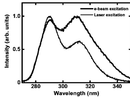
FIG. 4. E-beam and optically pumped fluorescence spectra. Compared with the optically pumped case in the same setup with a 262-nm optical pulse split from the photocathode excitation laser, the longer wavelength side of the spectrum is significantly enhanced.
