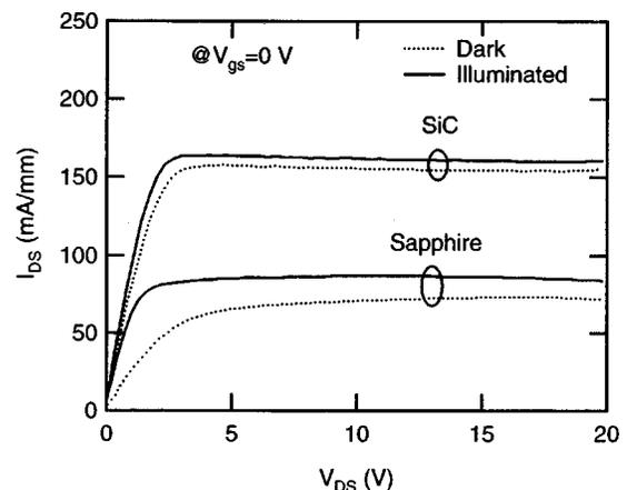
FIG. 4. dc  $I_{DS}-V_{DS}$  characteristics of AlGaIn/GaN HEMTs on sapphire and SiC substrates measured under dark and white-light illumination.
