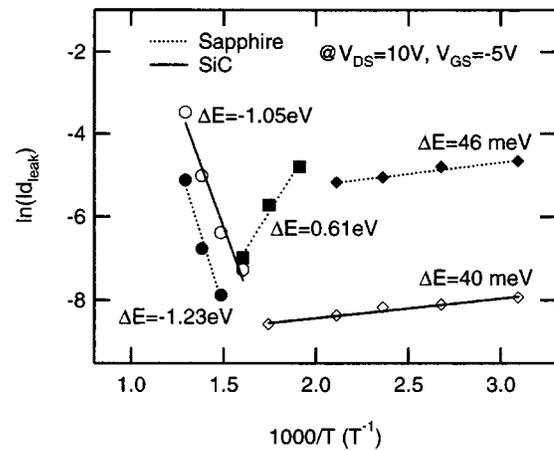
FIG. 3. Activation energy plot of drain leakage current ( $I_{DLeak}$ ) measured at the gate voltage of  $V_g = -5$  V and drain voltage of  $V_{DS} = 10$  V.
