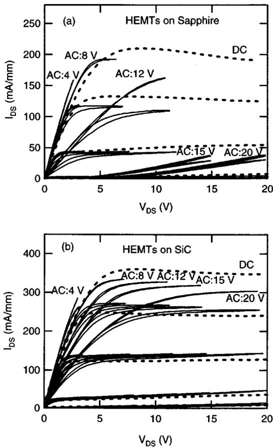
FIG. 1. Measured dc and ac  $I_{DS}-V_{DS}$  characteristics (for different drain sweep voltages  $V_{DS}=4, 8, 12, 15,$  and  $20$  V) of AlGaIn/GaN HEMTs on (a) sapphire and (b) Si-SiC substrates. Top trace was at  $V_{GS}=+1.5$  V step voltage was  $-1.0$  V.
