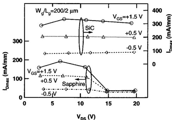
FIG. 2. Maximum drain current ( $I_{Dmax}$ ) of AlGaIn/GaN HEMTs on sapphire and Si-SiC substrates as a function of ac drain sweep voltages for different gate voltages ( $+1.5, +0.5,$  and  $-0.5$  V).
