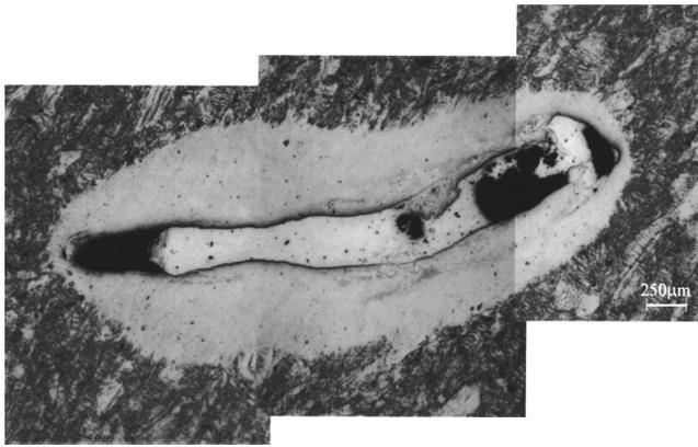
FIG. 1. Microstructure of the welded surface of specimen B, which was welded with a copper wire under the heat input power of 200 W s.
