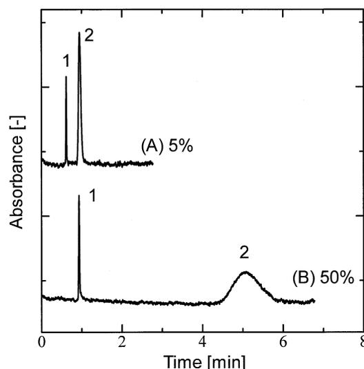
Fig. 2 Effect of the ODTES concentration on separation. Column: i.d., 30  $\mu\text{m}$ ; whole length, 20 cm; effective length, 10 cm; modified with (A) 5% and (B) 50% ODTES; eluent, methanol/10 mM phosphate buffer (30/70); applied voltage, 5 kV; detection, 210 nm; injection, 1 kV for 5 s. Peaks: 1, thiourea; 2, naphthalene.
