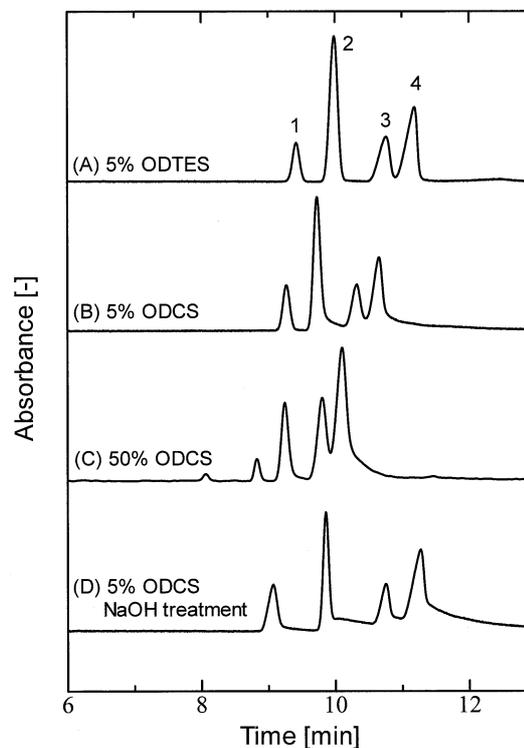
Fig. 4 Separation of neutral compounds by an ODSCS-modified OTCC. Column: i.d., 30  $\mu$ m; whole length, 40 cm; effective length, 28 cm; modified with (A) 5% ODTES, (B) 5% ODSCS, (C) 50% ODSCS, and (D) 5% ODSCS after a NaOH treatment. Other conditions are the same as in Fig. 1.
