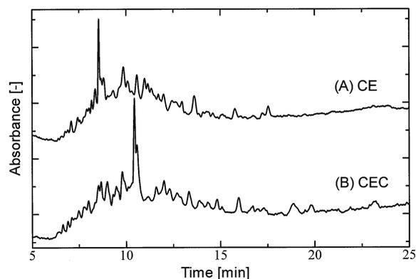
Fig. 5 Separation of proteins and peptides by CE and CEC. Column: i.d., 30  $\mu$ m; whole length, 40 cm; effective length, 28 cm; modified with 5% ODCS after a NaOH treatment; eluent, acetonitrile/300 mM phosphoric acid and 190 mM Tris (pH 2.1) (80/20); applied voltage, 15 kV; detection, 208 nm; injection, 10 kV for 5 s.
