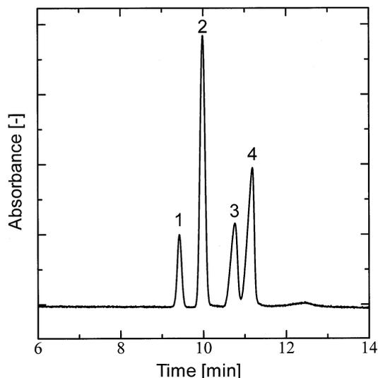
Fig. 1 Separation of neutral compounds by ODTES-modified OTCC. Column: i.d., 30  $\mu\text{m}$ ; whole length, 40 cm; effective length, 28 cm; modified with 5% ODTES; eluent, acetonitrile/10 mM phosphate buffer (30/70); applied voltage, 10 kV; detection, 210 nm; injection, 10 kV for 5 s. Peaks: 1, thiourea; 2, naphthalene; 3, biphenyl; 4, fluorene.
