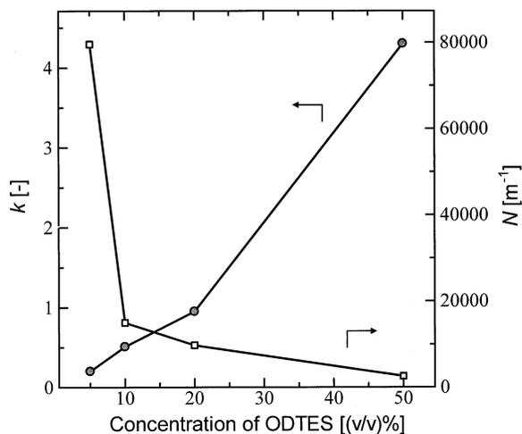
Fig. 3 Variation in the retention factor and theoretical plate number with respect to the ODTES concentration. Other conditions are the same as in Fig. 2.
