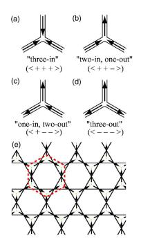
FIG. 3. (Color online) (a)–(d) Possible magnetization configurations at a vertex. (e) A kagomé lattice (solid lines) as Voronoi polygons of the vertices of the honeycomb lattice (dashed lines). Arrows represent magnetic moments. The dashed hexagon in (e) corresponds to the white or dashed hexagons in Figs. 2(a) and 2(b).
