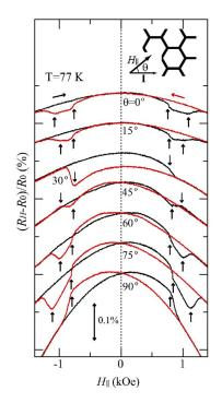
FIG. 4. (Color online) In-plane magnetoresistance curves of the permalloy honeycomb nanoscale network at 77 K.  $\theta$  denotes the angle between the magnetic field  $H_{\parallel}$  and the current I.  $R_H$  is the resistance between the Cu electrodes, which were placed at the edges of the sample.  $R_0$  is the resistance of the system in the absence of magnetic fields.
