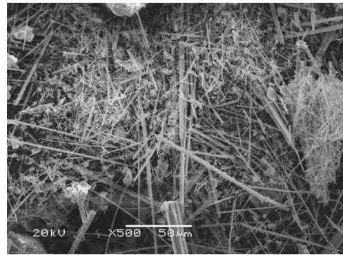
Fig. 2. SEM photograph of sprayed amosite.
