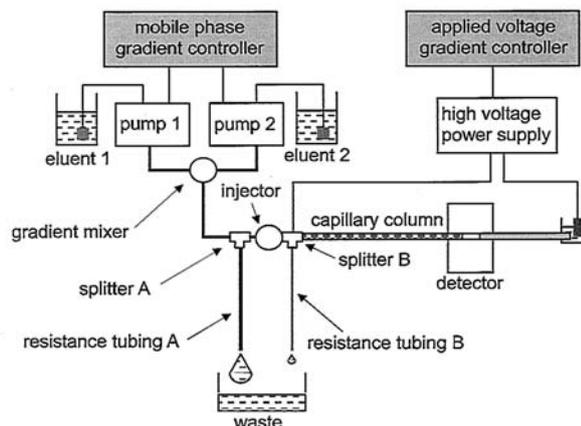
Fig. 1 Schematic diagram of dual-gradient capillary electrochromatography.
