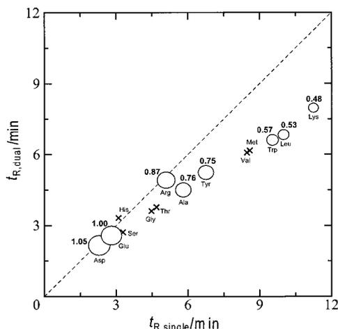
Fig. 4 Relationship between the elution time of amino acids with single and dual gradient. The size of the circle represents the relative half width ( $w_{1/2,dual}/w_{1/2,single}$ ), the values of which are given alongside the circle. The cross mark was used when either one or both half widths were not measured. The chromatographic conditions are the same as those in Fig. 3.
