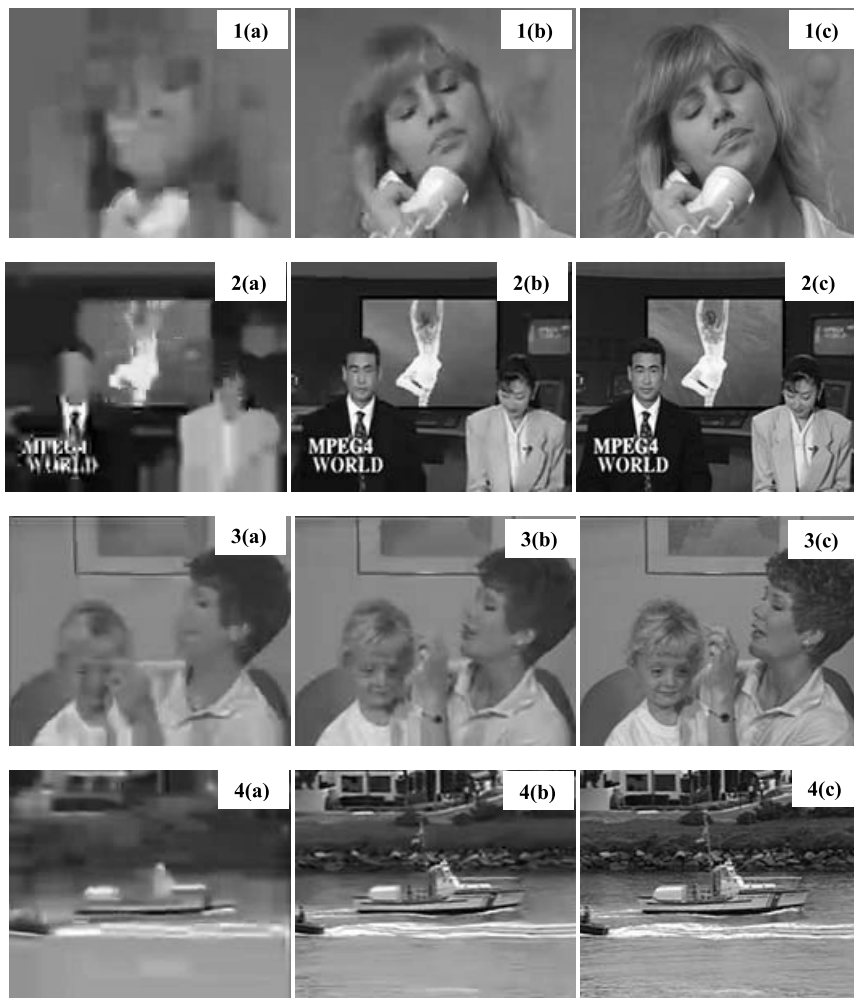
Fig. 11 Visual effect for burst error 40% frame loss for different video traces. The 135th reconstructed frame using Type 3: Spiral (1,2,3,4)a, Type 0:chessboard like pattern (1,2,3,4)b, and the proposed ECW FMO technique (1,2,3,4)c.
