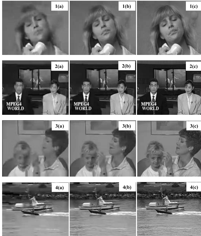
Fig. 10 Visual effect for burst error 20% frame loss for different video traces. The 45th reconstructed frame using Type 3: Spiral (1,2,3,4)a, Type 0:chessboard like pattern (1,2,3,4)b, and the proposed ECW FMO technique (1,2,3,4)c.
