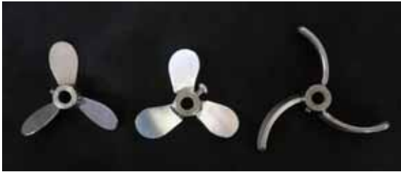
Fig. 2 Photograph of propeller and pfandler type impellers
