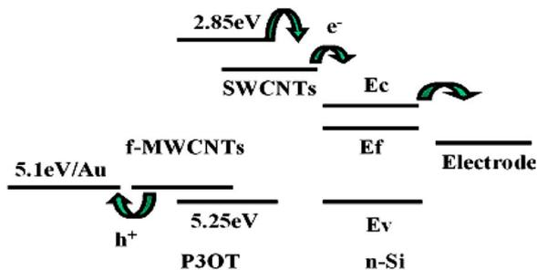
FIG. 4. (Color online) Energy band diagram of the fabricated device showing band alignment for *f*-MWCNTs and SWCNTs.
