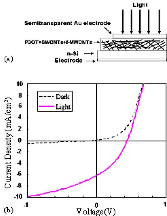
FIG. 2. (Color online) (a) Schematic of the P3OT/ $n$ -Si heterojunction solar cell incorporating  $f$ -MWCNTs and SWCNTs in the polymeric layer. (b) Current voltage ( $I$ - $V$ ) characteristic of the  $n$ -Si/ $f$ -MWCNTs+SWCNTs+P3OT/Au heterojunction solar cell in dark and under AM 1.5 simulated solar radiation. Cell is illuminated from the semitransparent Au electrode side.
