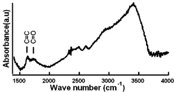
FIG. 1. FTIR spectrum of MWCNTs obtained after acid treatment.
