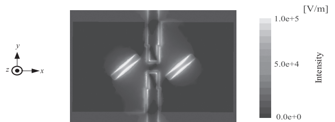
Fig. 3 Electric field intensity distribution in the xy -plane including the CC' -line.
