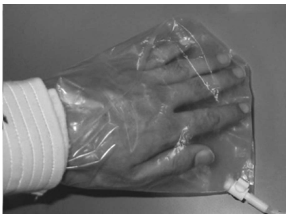
Fig. 1 Collecting device for skin gas emanating from hand
