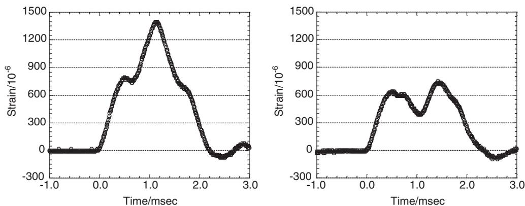
Fig. 2. Strain waveforms at the impact point with the backstop (a) for the small bowl (1) and (b) for the large bowl (2).
