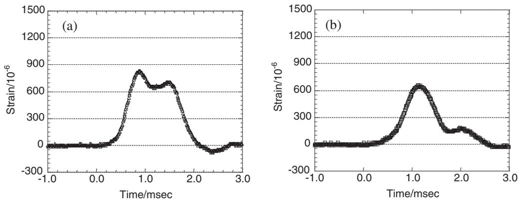
Fig. 3. Strain waveforms at the contact point with the backstop (a) for the small bowl (1) and (b) for the large bowl (2).
