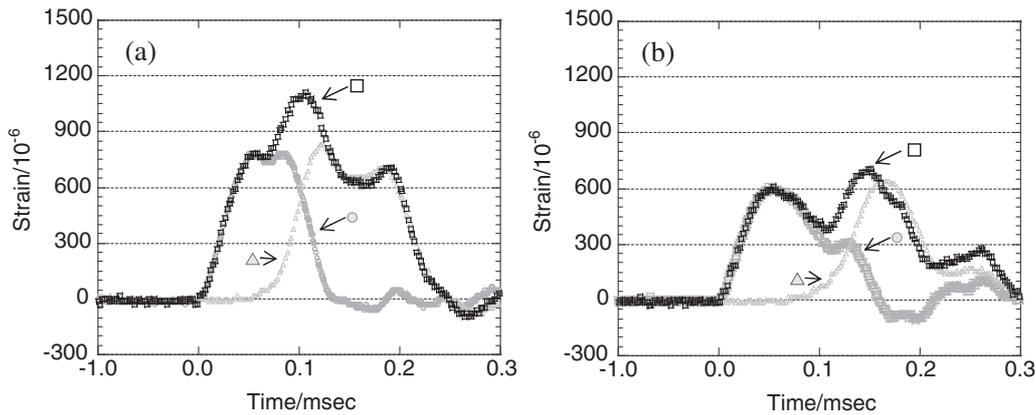
Fig. 7. Mechanism of two maximum peaks that appeared in the strain waveform: (a) small bowl (1); (b) large bowl (2). ●: strain waveforms caused by the initial impact, which are identical to the strain waveforms in Fig. 6. ▲: strain waveforms that returned from the backstop, which are equivalent to the strain waveforms in Fig. 3 after a delay of 0.35 ms for the small bowl (1) and 0.5 ms for the large bowl (2). □: strain waveforms estimated by the combination of ● and ▲.
