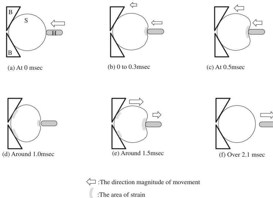
Fig. 5. Exaggerated illustration of the deformation of the large bowl (2) upon impact.
