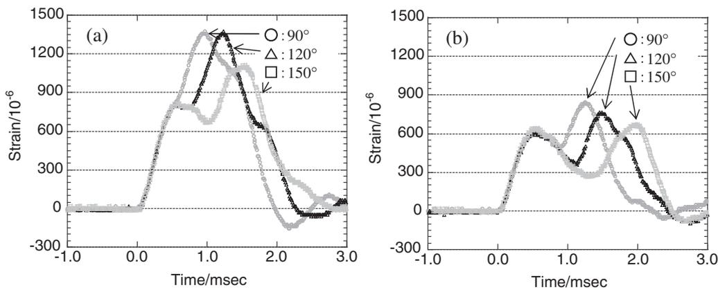
Fig. 8. Variation of the strain waveforms at the impact point with the open angle of the backstop ( $\alpha$ ): (a) small bowl (1); (b) large bowl (2).
