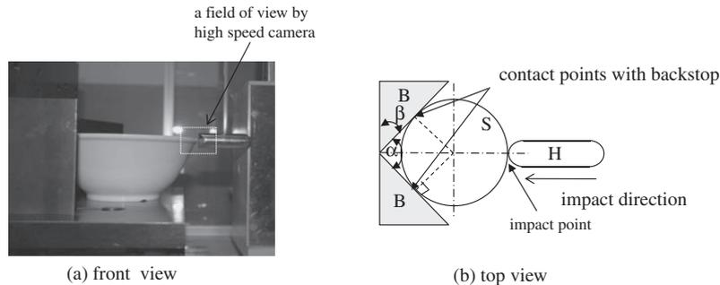
Fig. 1. Schematic diagram of the impact test: (a) front view; (b) top view (S: test specimen, B: backstop, H: hammer,  $\alpha$ : open angle,  $\beta$ : apex angle).
