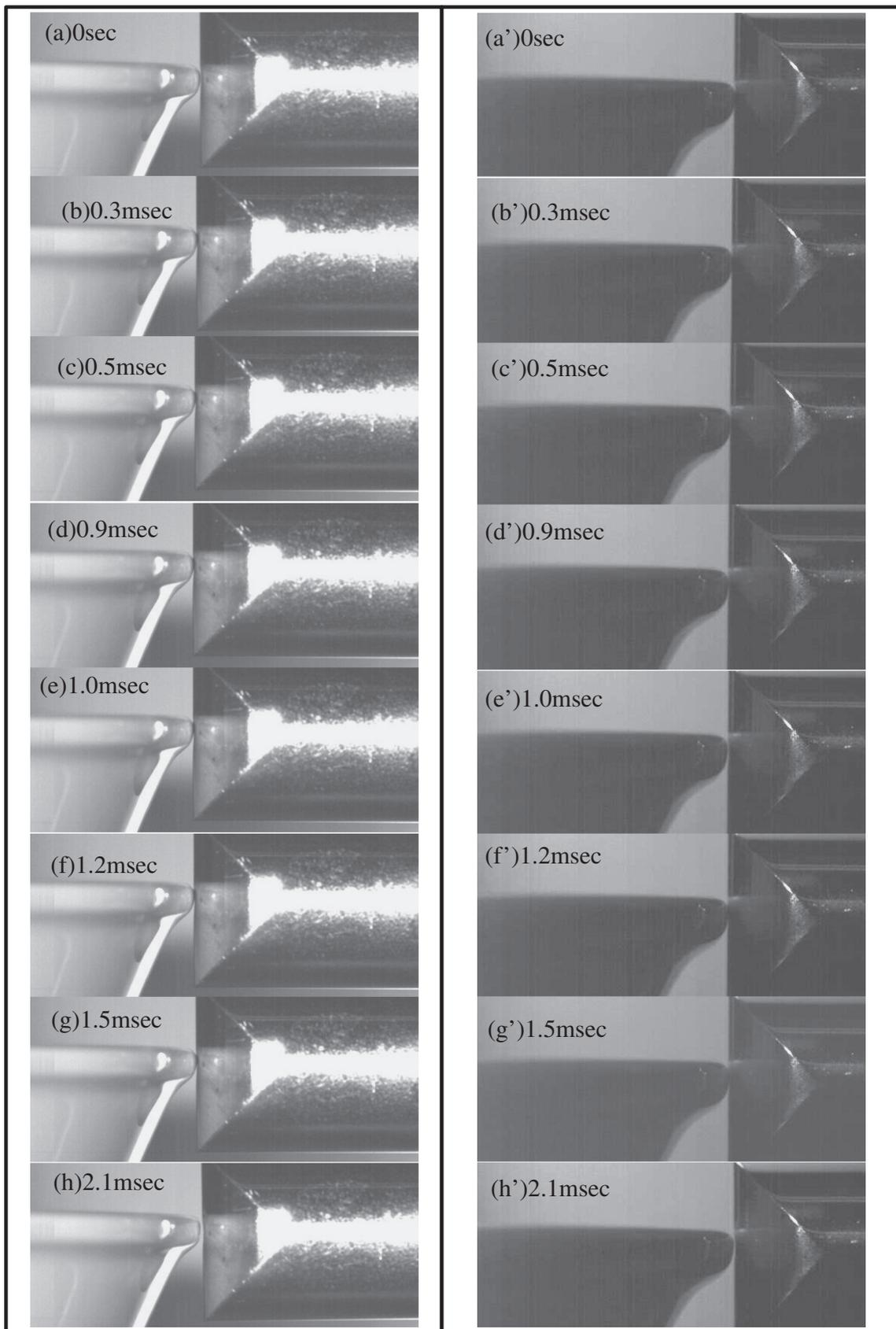
Fig. 4. Photographs of the bowl and hammer during impact captured by the high-speed camera: (a) through (h) small bowl (1); (a') through (h') large bowl (2).
