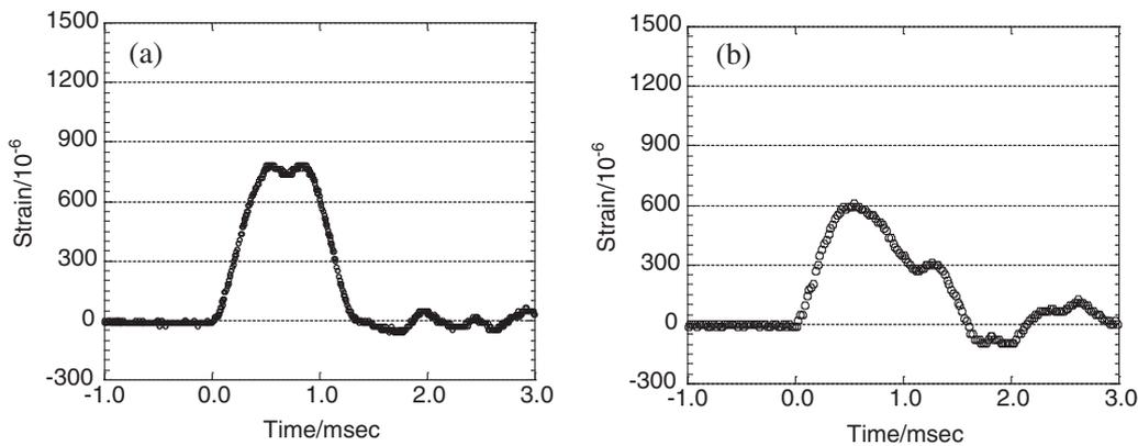
Fig. 6. Strain waveforms at the impact point without the backstop (a) for the small bowl (1) and (b) for the large bowl (2).
