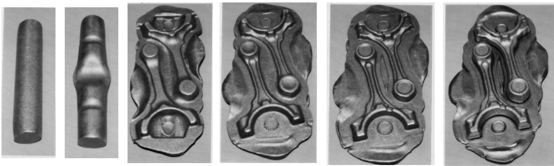
Fig. 2-1 Forging process of connecting rod.
