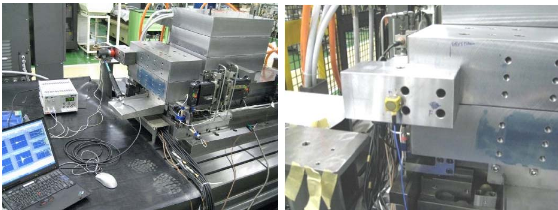
Fig. 3. 17 Compliance measurement in developed stage
