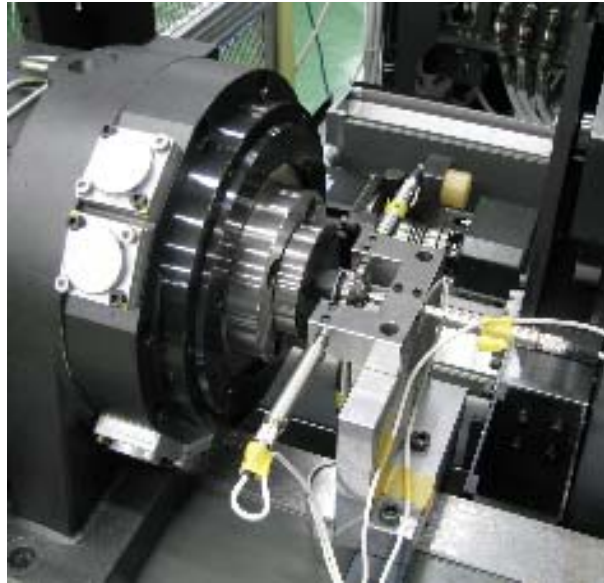
Fig. 4. 18 Experimental apparatus of rotational accuracy measurement
