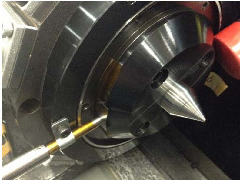
Fig. 4.14 Compliance measurement in radial direction
