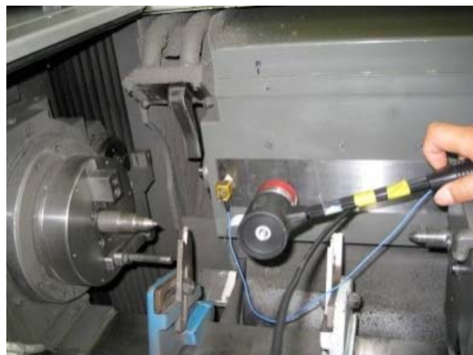
Fig. 3. 18 Compliance measurement in conventional grinding head
