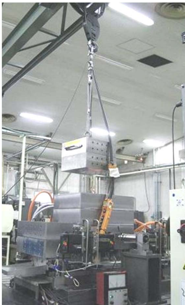
Fig. 3. 14 Static stiffness measurement in developed stage
