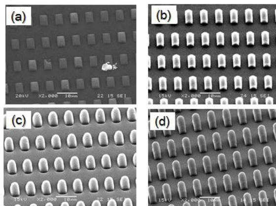
**Fig. 2** Surface morphology SEM images of the thermally nanoimprinted Nafion films under 24 MPa at (a) R.T., (b)  $110^\circ\text{C}$ , (c)  $140^\circ\text{C}$ , and (d)  $170^\circ\text{C}$ .
