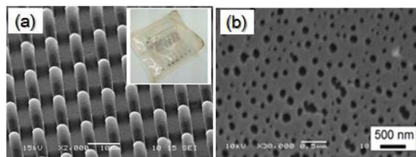
**Fig. 3** (a) SEM image of the imprinted Nafion under 24 MPa at  $200^\circ\text{C}$  using the Si mold and (inset) its optical photograph. (b) SEM image of the imprinted Nafion surface at  $170^\circ\text{C}$  using the novel quartz mold.
