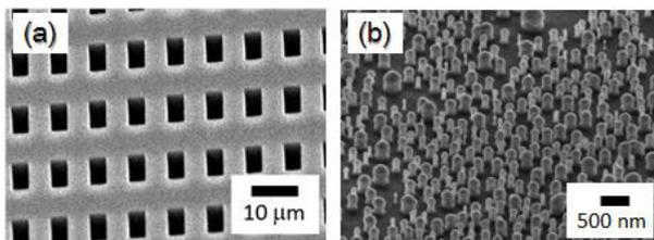
**Fig. 1** Surface morphology SEM images of (a) the Si mold with a  $5 \times 5 \mu\text{m}$  square pattern and (b) our novel 200 nm resolution mold used in this study.
