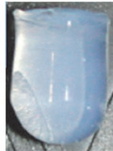
Fig.5 Appearance of silica aerogel prepared by solvent exchange treatment and by heat-drying at ambient pressure.
