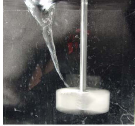
Fig.11 Photograph of surface vortex of six blade paddle impeller in rectangular vessel
