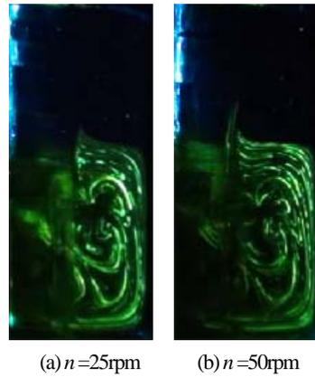
Fig.13 Comparison of streak line of Fullzone at  $Re = 100$
