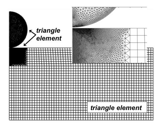
The mesh used for the finite element method.
