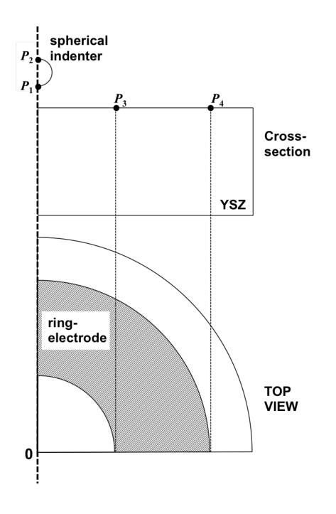
Cross-section and top views of the sample geometry for the FEM calculation.
