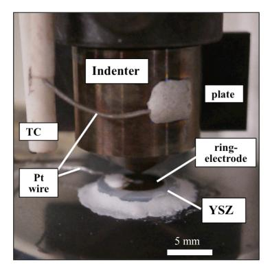
Photograph of the indenter and ring-electrodes for the high-pressure impedance test (TC: thermocouple, bar 5 mm).
