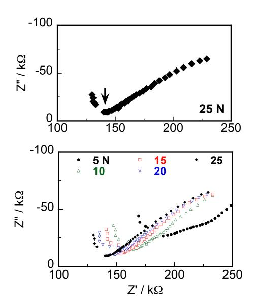
Cole–Cole plots of YSZ at 500 °C and 5 N for the ring electrode. The resistivity shown by the arrow (the first semicircle) was used for the calculation of conductivity.
