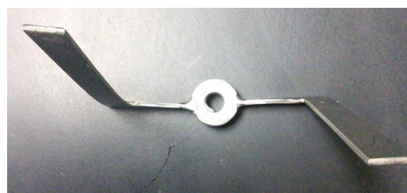
Fig.2 Broken anchor impeller
