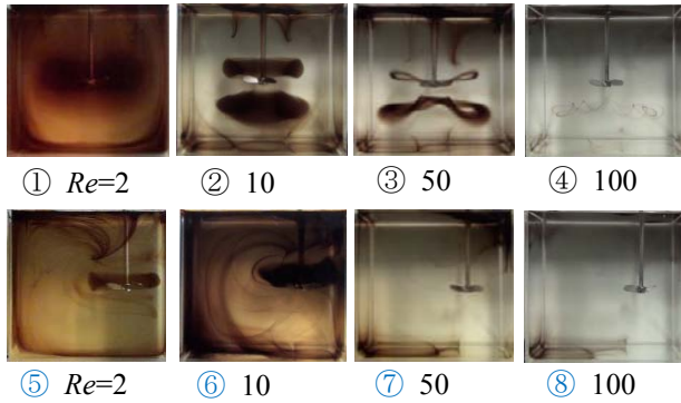
Fig. 20 Mixing patterns obtained with propeller impeller(5) in rectangular vessel in rectangular center mixing vessels ①-④ and in eccentric mixing vessels ⑤-⑧.
