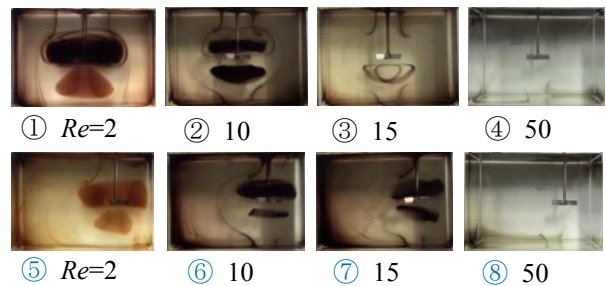
Fig. 18 Mixing patterns obtained with pitched paddle impeller(4) in larger rectangular center mixing vessels ①-④ and in eccentric mixing vessels ⑤-⑧.
