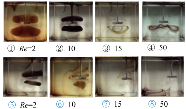
Fig. 16 Mixing patterns obtained with pitched paddle impeller(4) in larger rectangular center mixing vessels ①-④ and in eccentric mixing vessels ⑤-⑧.
