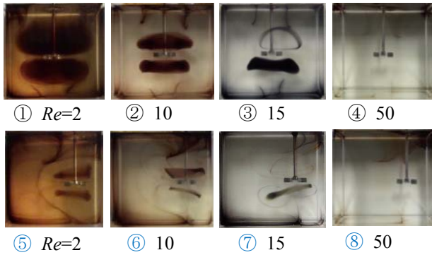
Fig. 12 Mixing patterns obtained with Rushton turbine(3) in rectangular center mixing vessels ①-④ and in eccentric mixing vessels ⑤-⑧.
