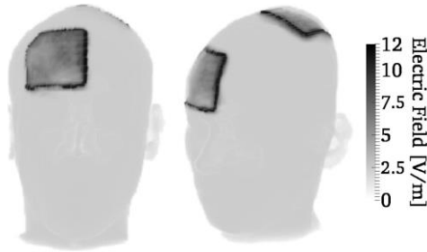
図 2 頭部内誘導電界強度の分布 Fig.2 Distribution of induced electric field in the head.
