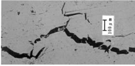
Fig. 7 The optical micrograph of the vertical cross-section of commercially pure iron specimen (sample No. N7) that indicates spall-damage to consists mainly of cracks. The image was taken after the first impact stress of 3.2 GPa.
