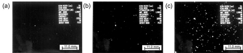
Fig. 5 The variation of spall-damage in commercially pure iron (sample No. N1) induced by consecutive impacts during repeated testing with the second impact stress (1.8 GPa) lower than the first one (3.5 GPa). The C-scan images taken at the depth of 3.0 mm below the impact surface illustrate the scenario after the first (a), second (b) and third (c) impact, for which the applied impact stress equaled 3.5, 1.8 and 3.5 GPa, respectively.
