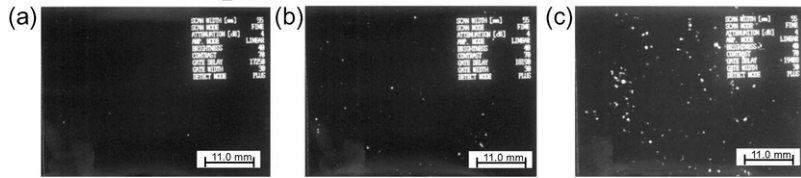
Fig. 4 The variation of spall-damage in commercially pure iron (sample No. N4) induced by consecutive impacts during repeated testing with the second impact stress (3.8 GPa) higher than the first one (2.8 GPa). The C-scan images taken at the depth of 3.5 mm below the impact surface illustrate the scenario after the first (a), second (b) and third (c) impact, for which the applied impact stress equaled 2.8, 3.8 and 4.9 GPa, respectively.
