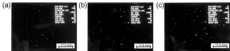
Fig. 6 The variation of spall-damage in commercially pure iron (sample No. N17) induced by consecutive impacts during repeated testing with the second impact stress (2.4 GPa) lower than the first one (3.6 GPa). The C-scan images taken at the depth of 3.0 mm below the impact surface illustrate the scenario after the first (a), second (b) and third (c) impact, for which the applied impact stress equaled 3.6, 2.4 and 2.2 GPa, respectively.
