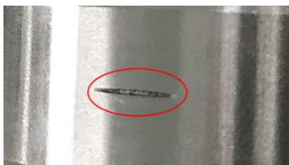
Figure 8.2 Bearing with a scratch 5 mm.
