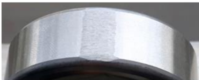
Figure 8.3 Abrasion bearing sample.
