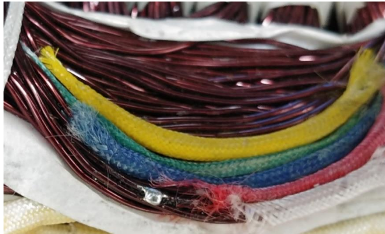
Figure 7.4 Short-circuit insulation failure.
