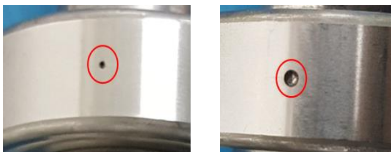
Figure 4.2 Bearing with a hole 0.5 mm (left) and hole 2 mm (right).
