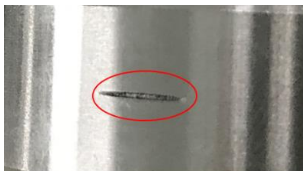
Figure 7.2 Bearing with a scratch 5 mm.
