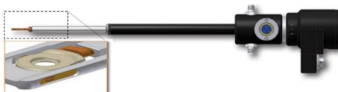
Figure 2.9: Heating holder for in situ experiments [10].
