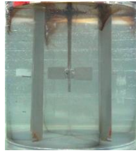
Fig. 5 Mixing pattern of larger vessel at Re=30 ( nt=300 , D=0.36 m)
