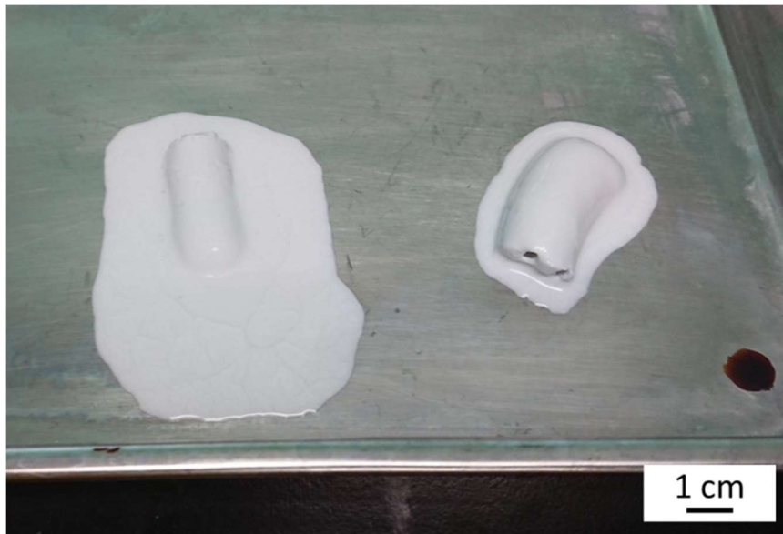
Fig.2-9 Photograph of porous alumina bodies with added 2.7 g ethanol, immediately after rapid freezing process for 5 min and removing the cylindrical mold.
