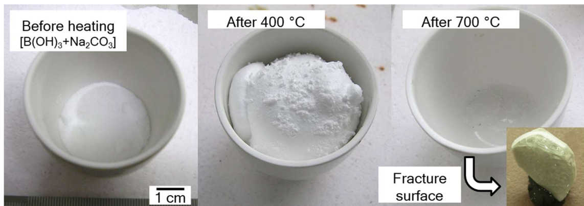
Fig.3-17 Form change accompanying heating of flux powder ( \text{B}(\text{OH})_3+\text{Na}_2\text{CO}_3 ).
