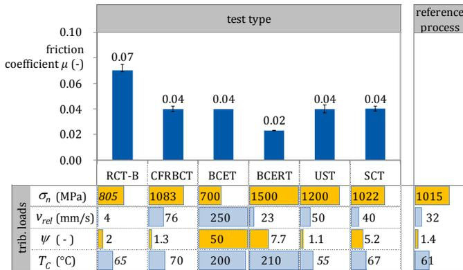
**Figure 3.** Friction coefficients and tribological loads of the friction tests and the reference process.
