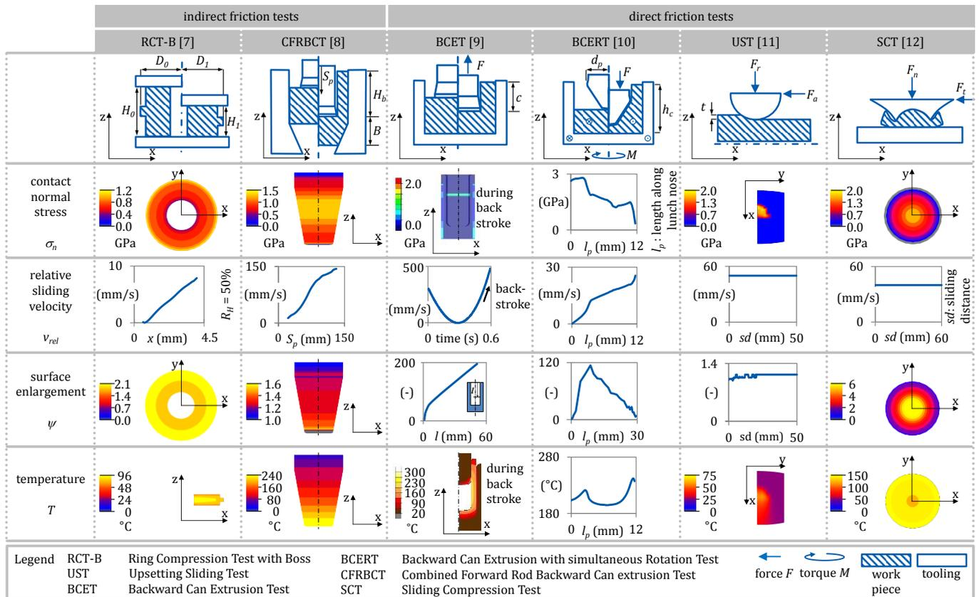
**Figure 2.** Comparison of tribological loads of the investigated friction tests.
