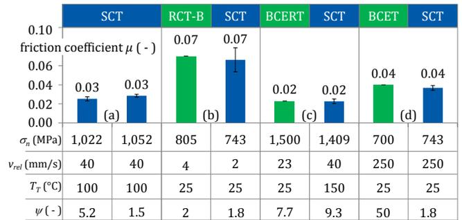
**Figure 4.** Friction coefficient as a function of the tribological loads, determined with the SCT, in comparison to the RCB-T, BCERT, and BCET.
