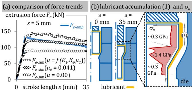
**Figure 5.** Comparison of extrusion forces  $F_e$  (left) and schematic depiction of lubricant accumulation and  $\sigma_n$  (right).
