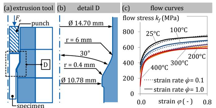
Figure 1. Tool geometry of reference forming process ( $F_e$ : extrusion force, a), detail of forming die (b), and experimentally determined flow curves.
