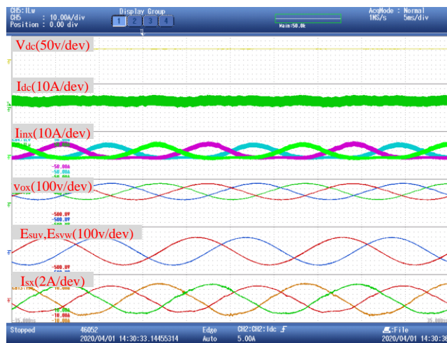
Figure 4.9: Experimental results of proposed SEPIC-BDI at case 2.
