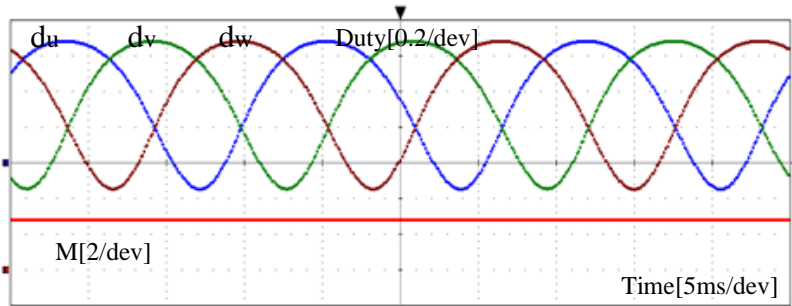
Figure 4.14: Duty cycle and Static gain M of proposed differential inverter.
