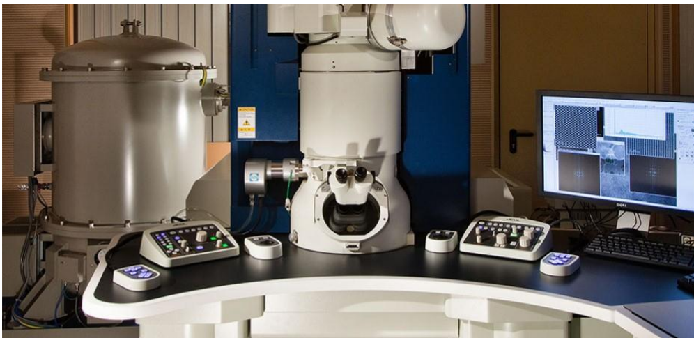
Figure 2.8: TEM model: JEM-ARM200F (JEOL) used in the thesis [17].
