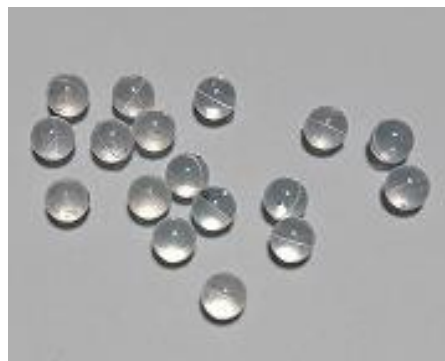
(b) Material: silicone elastomer TSE3466, diameter of particles: 4 mm
