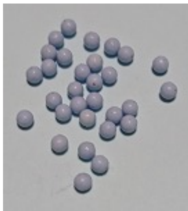
Fig. 3.2 Photographs of particles. Material: silicone rubber TSE3453, diameter of particles: 3 mm
