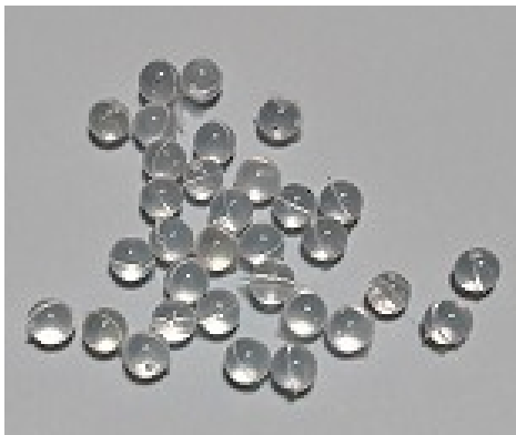
(a) Material: silicone elastomer TSE3466, diameter of particles: 3 mm
