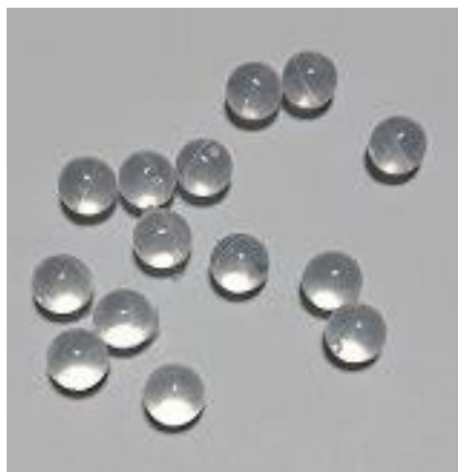
(c) Material: silicone elastomer TSE3466, diameter of particles: 5 mm
