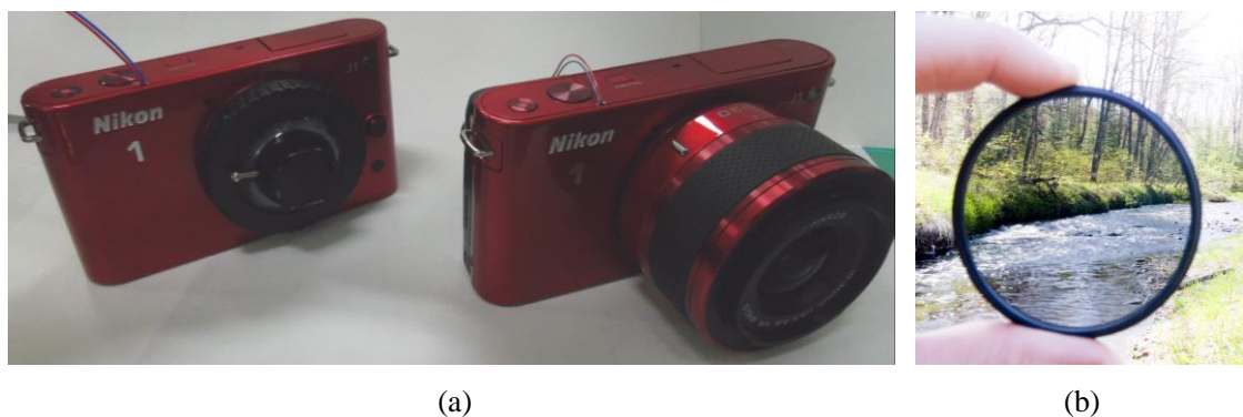
Fig. 1.21 (a) Digital mirrorless single-eye camera (modified camera (left), commercial camera (right)), (b) Neutral-density (ND) filter.
