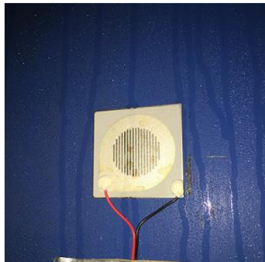
Photo 3.2 ACM sensor on the web of girder
