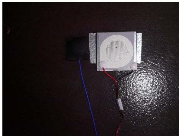
Photo 5.3 ACM sensor on the flange of girder at point B.
