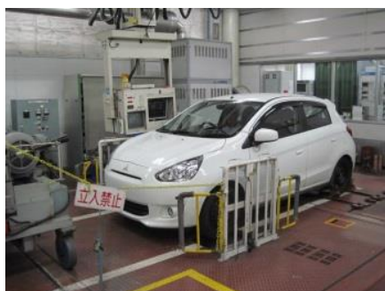
A) Chassis Dynamo Test
