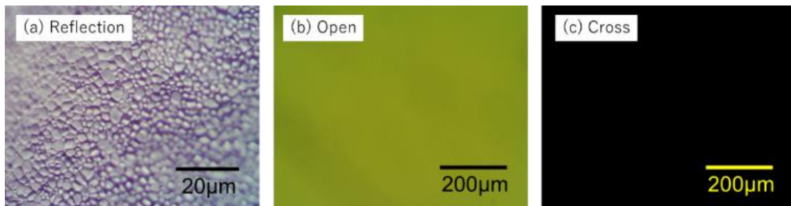
Figure 5.3 (a) Reflection, (b) transmission (open nicol) and (c) transmission (crossed nicol) polarizing optical micrographs of \text{Dy}_2\text{O}_3 ceramics.
