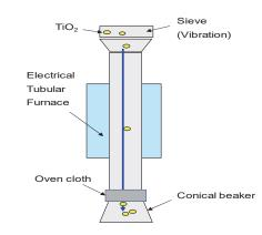
Fig. 1 Outline of the natural dropping thermal treatment
