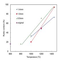
Fig. 3 Rutile conversion ratio for P25
