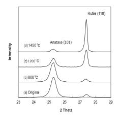
Fig. 2 XRD patterns of thermally-treated P25
