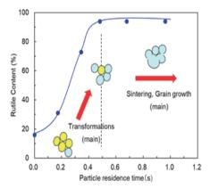
Fig. 4 Illustration of thermal treatment based on particle residence time
