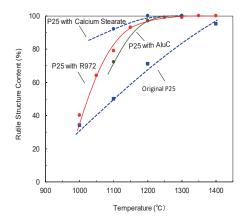
Fig. 7 Rutile conversion ratio for thermally-treated P25 mixed with external additive
