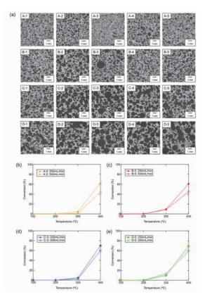
**Figure 7.** (a) Pore structure of fabricated hydroxyapatite filters observed by X-CT. (b–e) Catalytic decomposition of ethyl acetate using the selected filters in (a). (Reprinted from Scientific Reports 2021, 11, 7512. Copyright © The Authors(s) 2021.).
